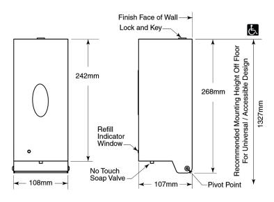
Model WA7025 is our wall mounted automatic liquid soap dispenser. Manufactured from grade 304 stainless steel with a satin finish. Supplied with refillable 0.85 litre plastic soap container and lockable hinged housing. No-touch sensor operation with battery supply.
